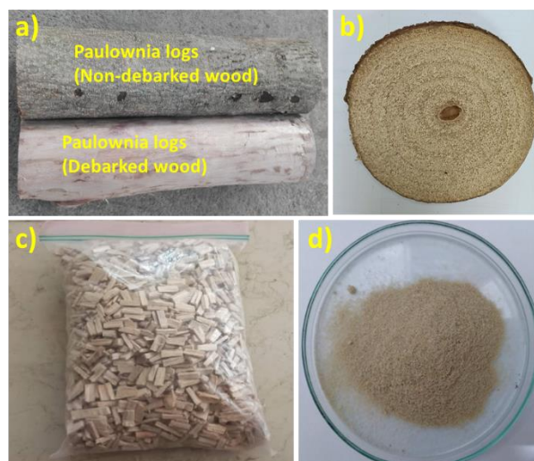
Figure 1. Preparation steps of Paulownia wood for chemical analysis. a) tree logs, b) a wood disc, c) wood chips, and d) wood powder.
