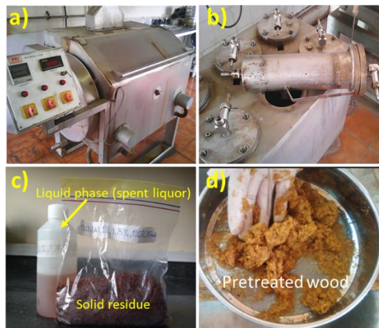
Figure 2. a) Electrically heated laboratory glycerol bath, b) 2.5 L steel cylinders, c) Paulownia wood after acid pretreatment, and d) pretreated Paulownia wood after the washing stage.
