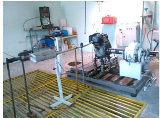
Figure 3. Performing engine performance tests with a dynamometer
