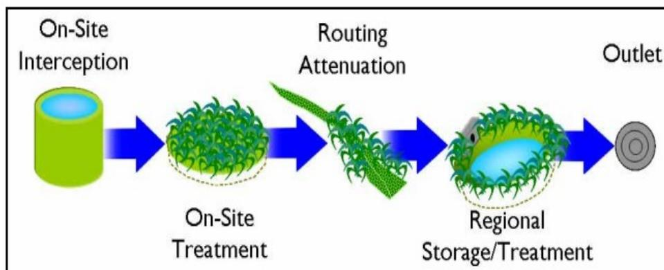
**Figure 4.** A schematic of complete GI treatment for runoff control (Shoemaker et al., 2009)
