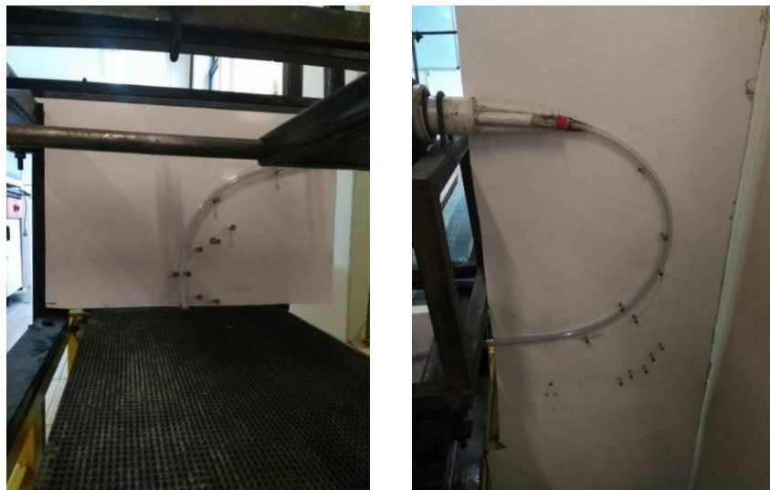
Figure 2. The seed tube and grease belt constructed for the experiments. A light-sensitive displacement sensor was installed at the beginning of the tube, while another sensor was installed at the end of the tube to investigate the movement of the seeds in the tube. The sensors' data were transferred to a computer using an A/D converter for further analysis. An example of the output of the transmitter-receivers used in the seed tubes with different curvature radii is depicted in Figure 3. As shown in the figure, the movement of the seeds in the seed tube is affected by its curvature shape.
